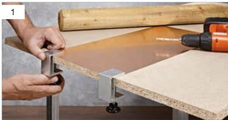
If you want to bend a metal sheet to form a rounded structure, round timber in different diameters is the perfect solution. For the sheet to be bent exactly parallel, it must not slip during the powerful bending process. To this end, you must ensure that it is firmly clamped on the edge of the workbench (e.g. with **alfer**<sup>®</sup> multi-clamps or other vices).
