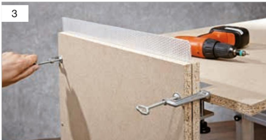
Use the **alfer**® multi-clamp to tightly clamp the sandwiched structure in front of the workbench.
