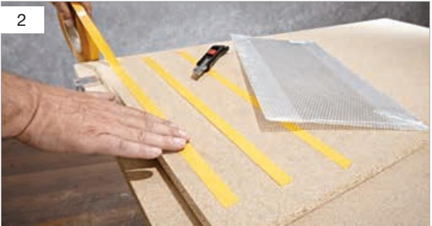
Tape the sheet with the protective cover onto a particle board with the bending edge lying precisely along the edge of the board. Next, place the second particle board flush with the bending edge and screw the two boards together outside the sheet.
