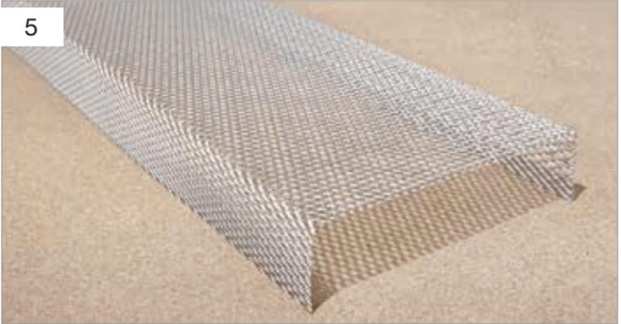
This image shows you the finished U-sheet. It is precisely flush, parallel and rectangular.
