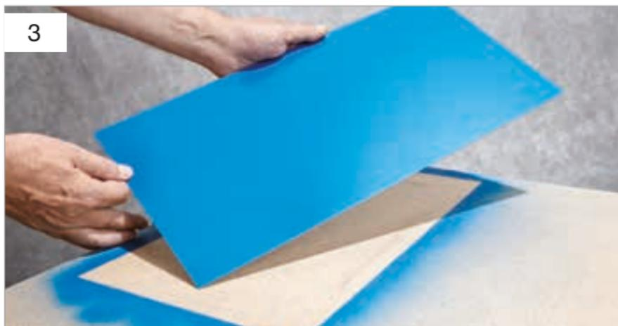
Tip: for the best results, apply the paint in multiple stages, leaving it to dry for at least 5 minutes between each application. This prevents paint runs and provides optimal paint coverage.
