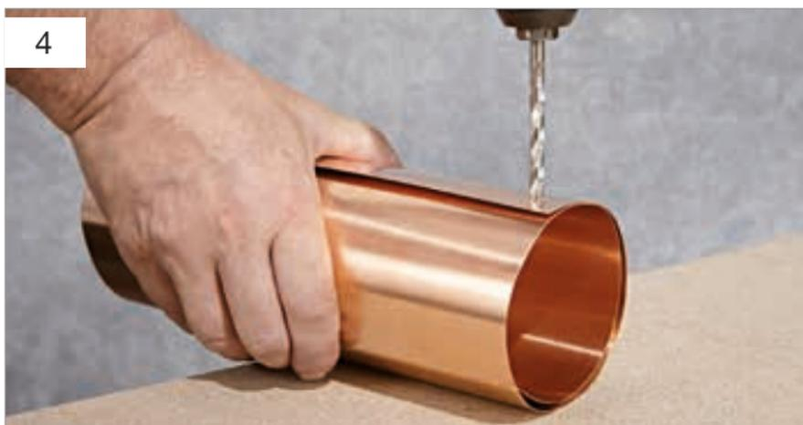
You can now push the sheet into itself until you have created the precisely desired diameter. Next, fix this diameter by riveting, soldering, bonding or welding the sheet.
