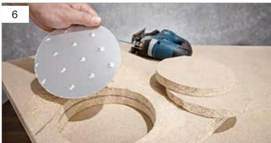
Here, you can see the perfectly round, non-scratched circular piece of the round studded sheet. Even on the studs, the jigsaw has not slipped from the cut line thanks to the guidance from the particle boards.
