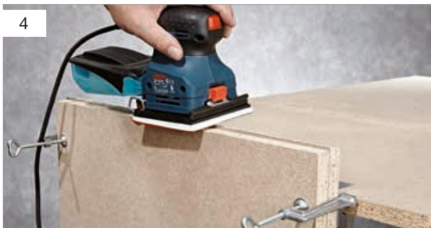
When sanding a very rough sheet edge, we recommend first using very coarse-grained abrasive paper with a high material removing effect. Sand the sheet until it has the smooth edge that you desire.
