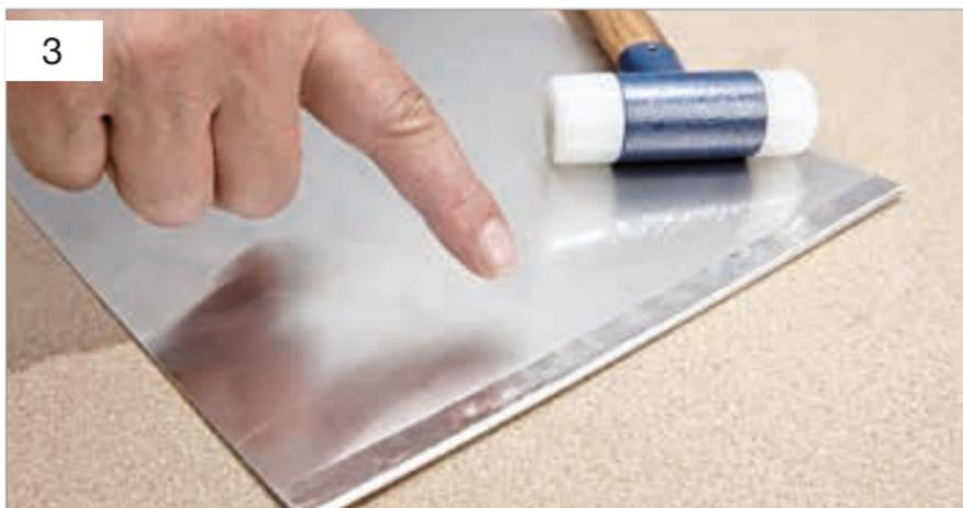
Next, anchor the sheet flat to the workbench and carefully tap down the short strip of sheet along its full length. The small sheet deformations do not impair the appearance of the finished product as they are on the underside of the sheet.
