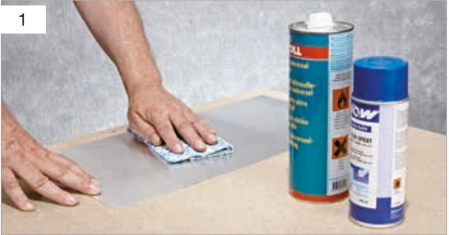
Metal sheets can be successfully painted. We recommend car spray paints because they ensure a uniform coat of paint and good bonding. Before painting, the sheets must be clean, free of grease and dust and totally dry. The sheet to be painted and the can of spray paint must also be at room temperature.
