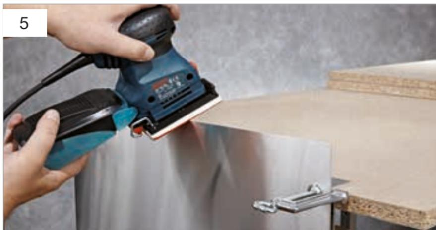
For the final smoothing stage, remove the sheet from the sandwich and clamp it without the particle boards. Next, attach finely-grained abrasive paper to the orbital sander and move it over the sheet edge again at a flat angle.
