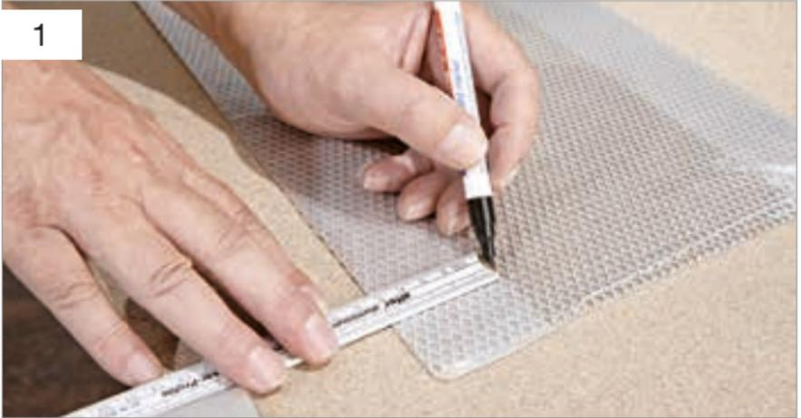
For straight bends, start by drawing your bending edge. We recommend leaving the protective cover on the sheet. This provides it with optimal protection and helps prevent it from being scratched while you work.
