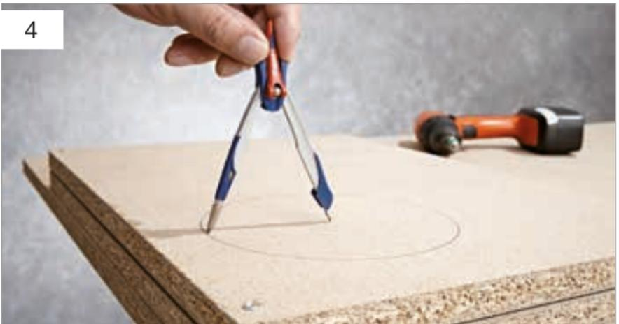
Next, draw clearly visible circles, straight or curved cut lines on the particle board without leaving any annoying marks on your sheet.
