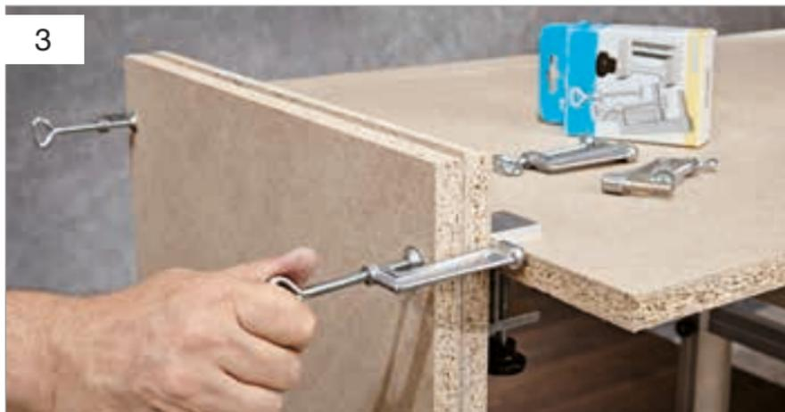
Clamp the 'sandwich' vertically in front of the workbench (ideally using an **alfer**® multi-clamp) and guide the orbital sander evenly along the protruding sheet at high speed.
