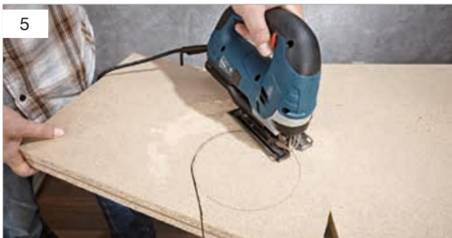
Now use the jigsaw to cut out your desired shape. We recommend working with a low stroke rate.
