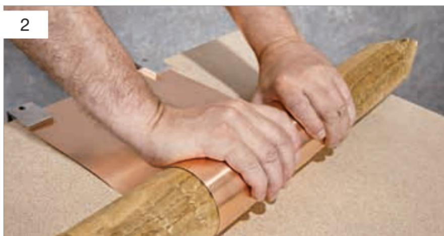
Always ensure that an exact right angle is formed with the longitudinal axis of the round timber! Next, roll the round timber towards yourself evenly and with a relatively high amount of force while also pushing it away from yourself, keeping it under pressure. Make sure that you roll the round timber in a straight line, so that the round body formed by the sheet is not spiral shaped. You can
