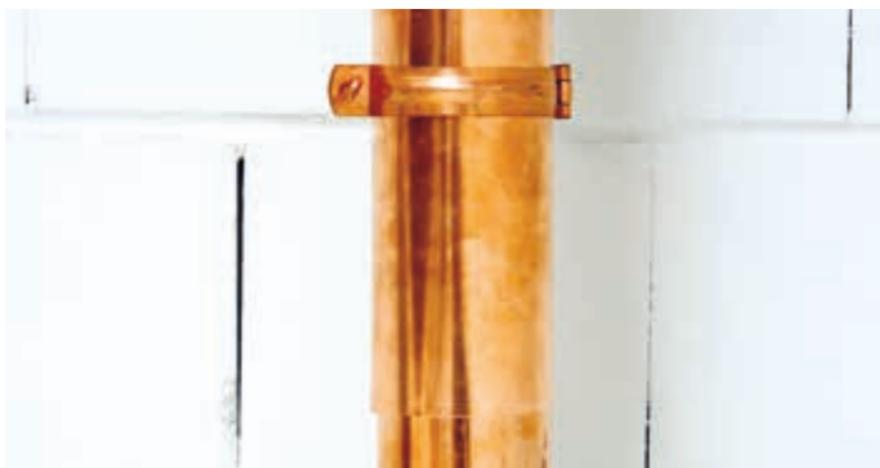
Cylindrical bend of a copper sheet.
