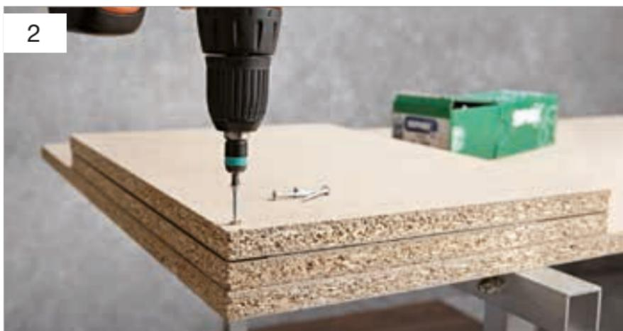
Screw or clamp the sheet between two particle boards in sandwich format (as in the cutting instructions above), ensuring that the uneven, rough edge of the sheet only protrudes 2–3 mm outside the particle boards. This reliably prevents the sheet from wobbling, bending or becoming scratched.
