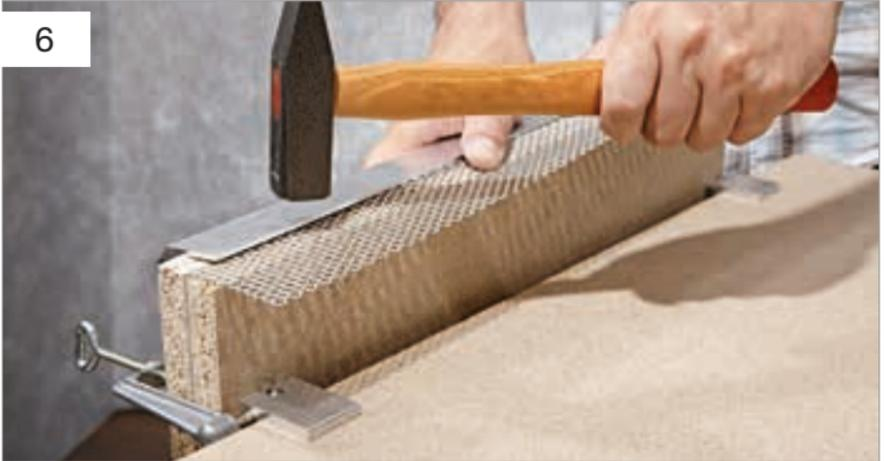
If you are unable to create the bend manually due to the sheet being too long (over approx. 80 cm) or too thick, you can also use a hammer and impact shield (profile or wood batten) to assist you and carefully tap the sheet down.
