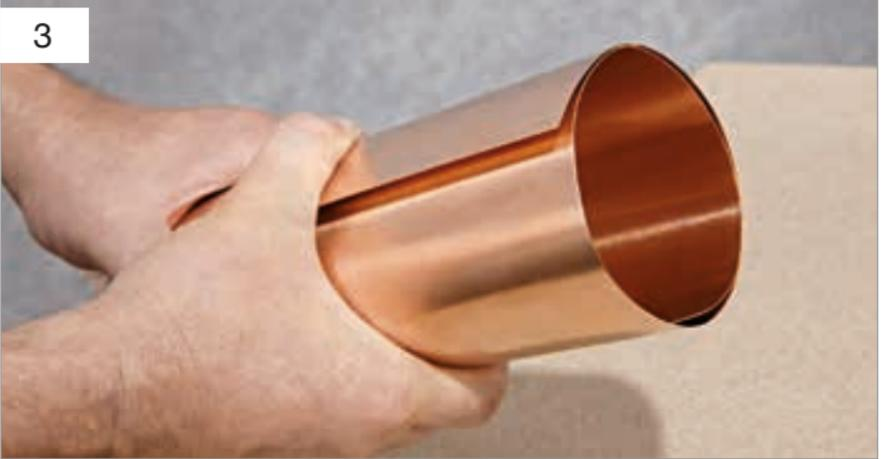
check this straight course by ensuring that the rolled sheet edge is always precisely aligned with the edge of the sheet still lying flat. Due to the spring recoil of the sheet you must rotate it about 1.5 times. On unrolling the round timber, the diameter of the bent sheet will expand by approx. 30%.
