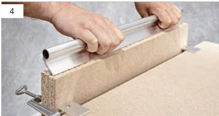
For the subsequent bend we recommend using a profile, roof strip or board to bend the projecting sheet forwards (towards the body) as uniformly as possible until it reaches the desired bend angle. If you do not want to bend just one angle, but rather create a U or Z-shaped sheet, simply repeat the process on the other side of the sheet.
