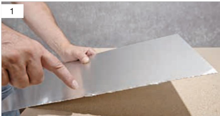
Professional tip: uneven, rough or even frayed sheet edges can be easily smoothed off lengthwise with an electric orbital sander. This applies to not only aluminium sheets but also steel ones.
